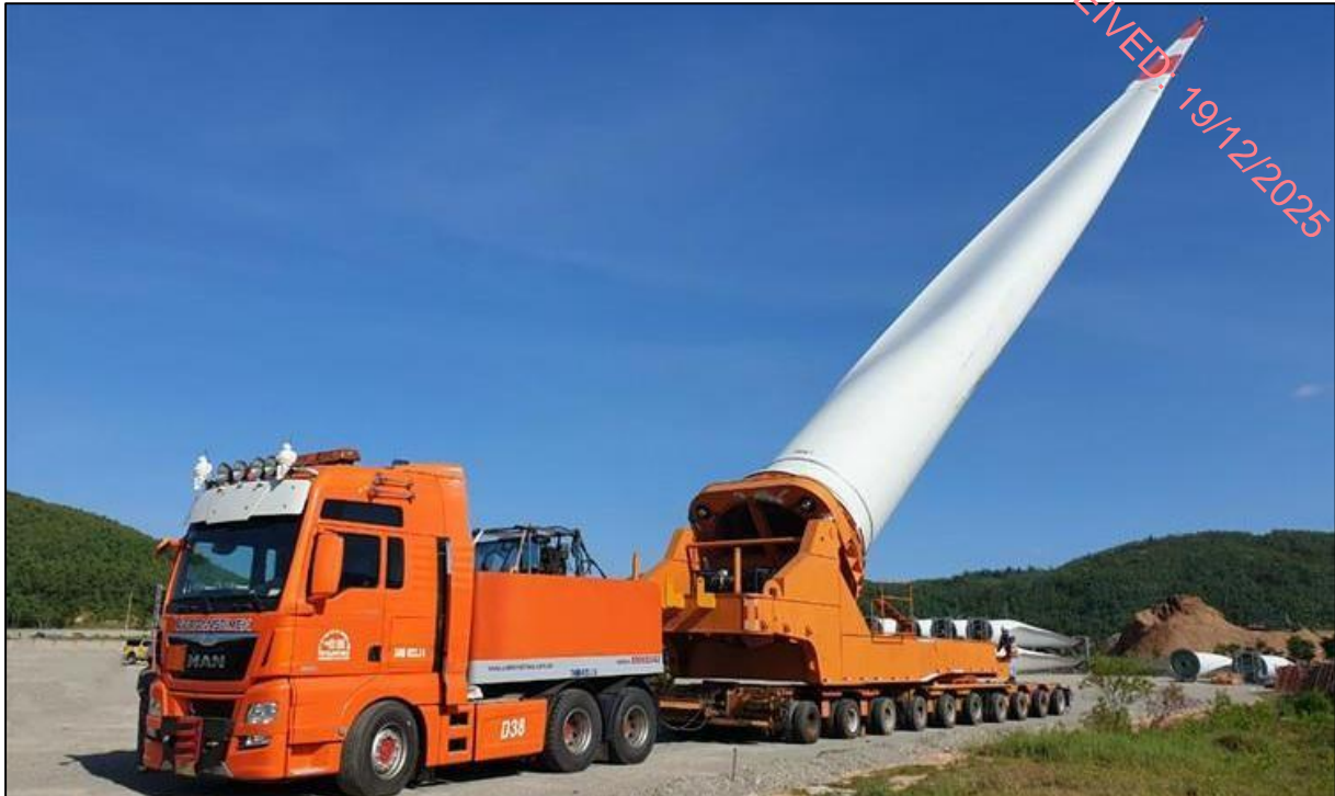
Figure 2-1: Blade Lifter Trailer with Blade Tilted to 60° from Horizontal
