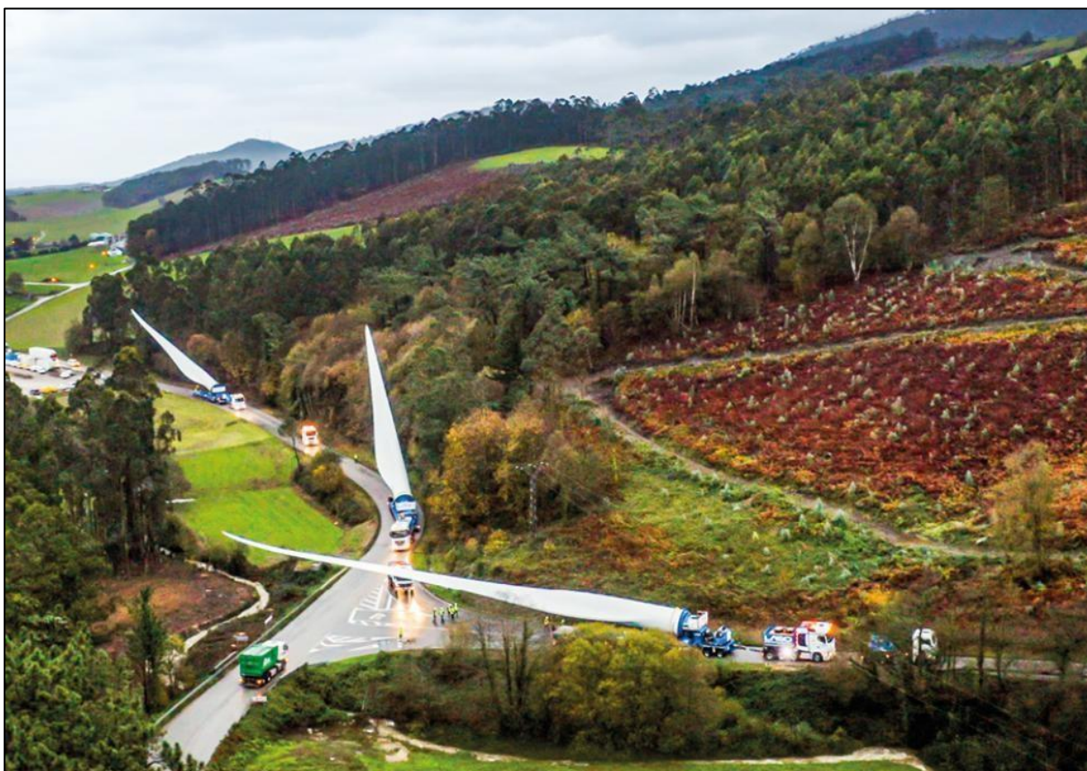
Figure 2-2: Blade Lifter Trailers in Convoy Transitioning from Tilted to Lowered to Avoid Overhead Line
