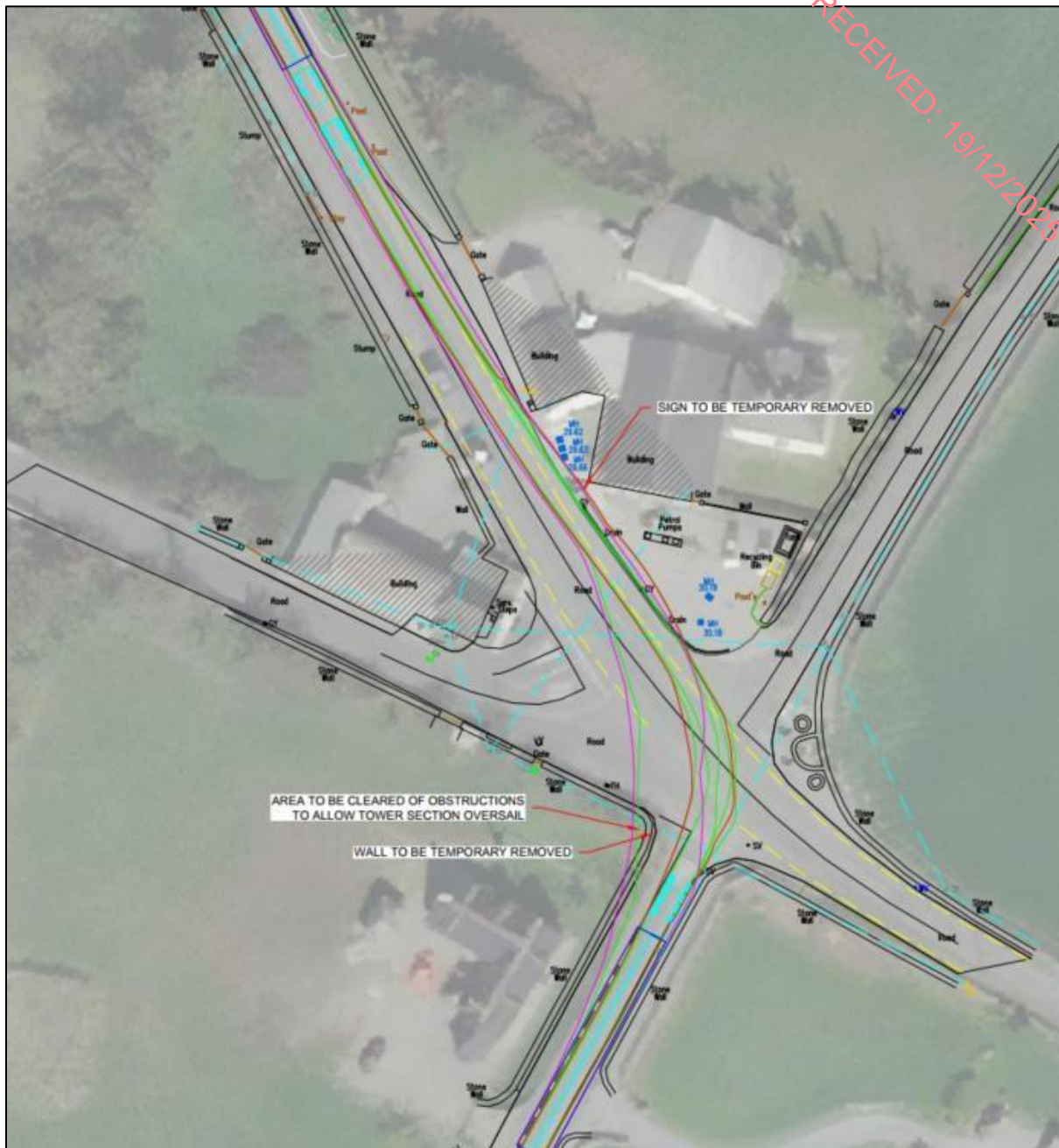
Figure 4-17: Swept Path Analysis of Pinch Point 7 (Obstructions)
